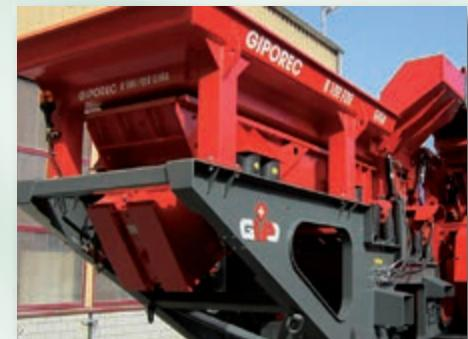
Hydraulic aggregates are widely used to drive unbalance excitors.
